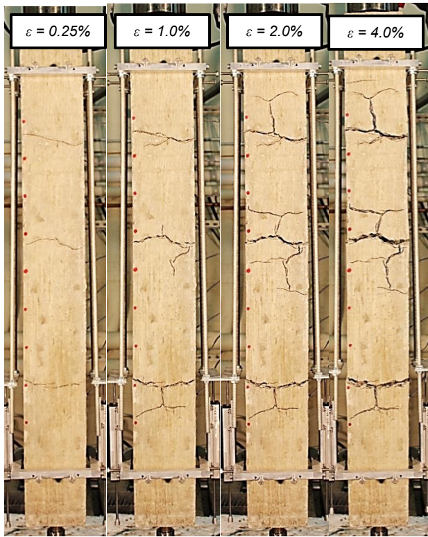
Figure 27. Cracking and strain distribution in specimen NC-12-127-sg
