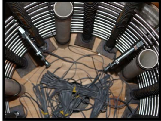
Figure A. 9. Coupler embedded in the column for threaded rods.
