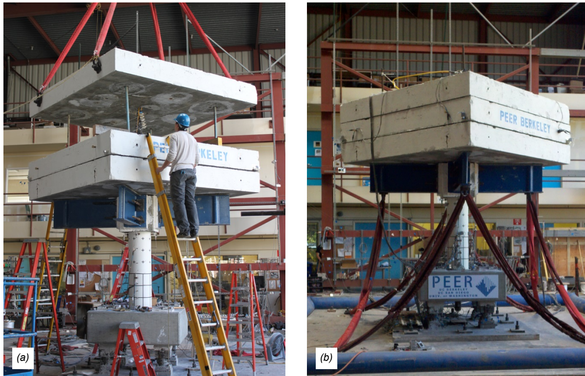
Figure 55. Photos during test preparation; (a) installation of the RC mass plates, (b) final test configuration prior to testing.
