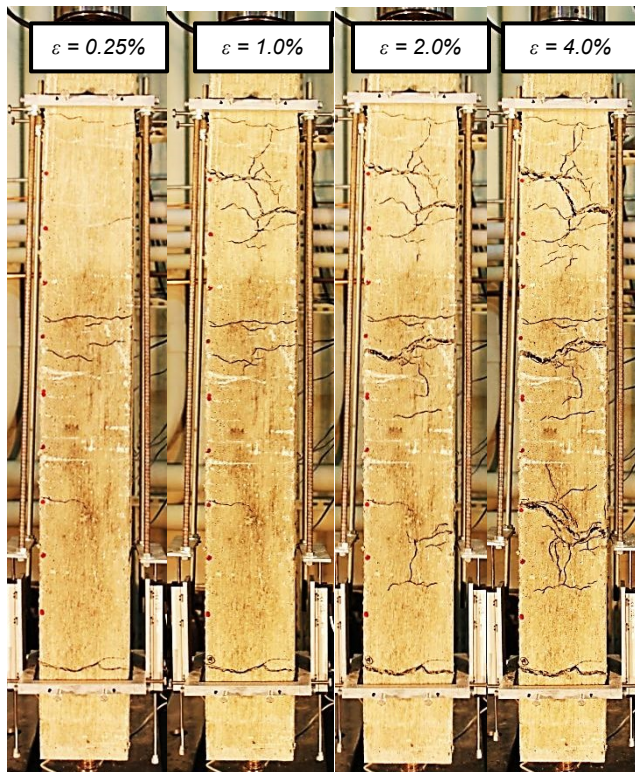
Figure 25. Cracking and strain distribution in specimen H-12-127-sg
