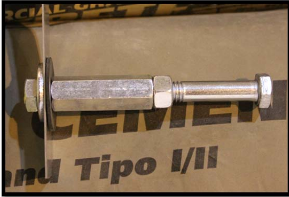
Figure A. 9. Coupler embedded in the column for threaded rods.
