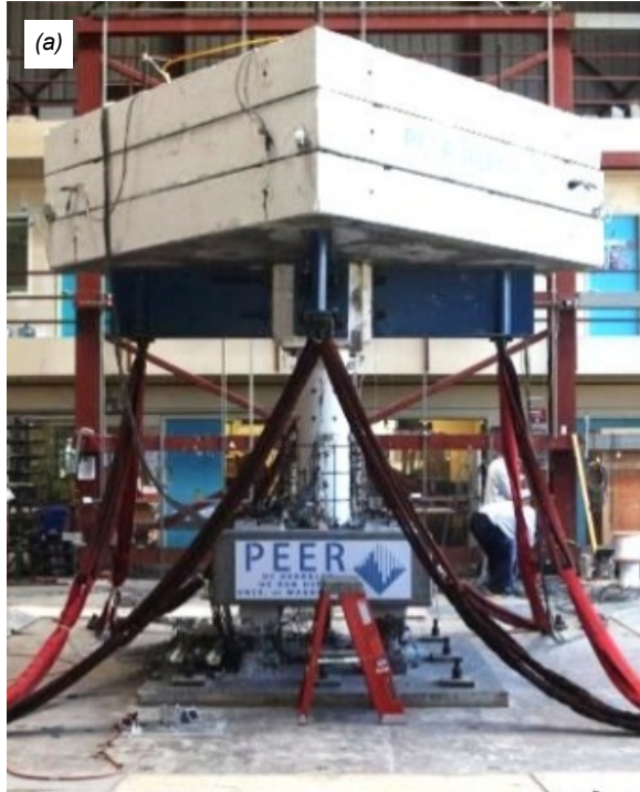
Figure 59. Elevation of columns at the end of testing; (a) PT HyFRC column with a residual drift ratio of 0.9% and (b) reference column with a residual drift ratio of 6.8%.
